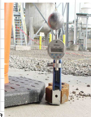
54-8 Electronic Dial Gage Telltale with 3-Pound Lead Weight
