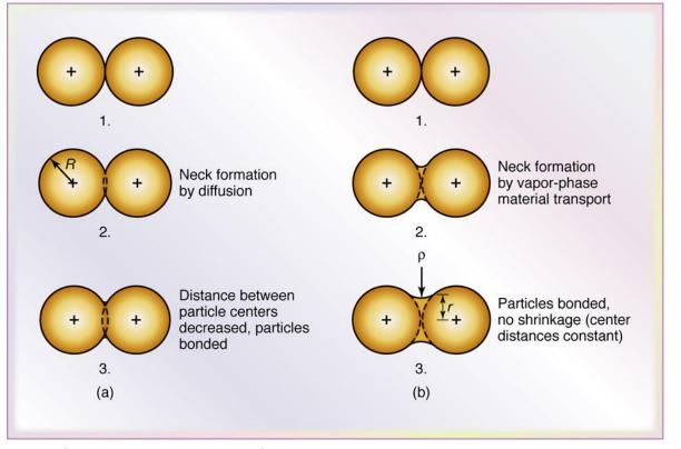
Schematic illustration of two mechanisms for sintering metal powders: (a) solid-state material transport; and (b) vapor-phase material transport. R = particle radius, r = neck radius, and p = neck-profile radius.
