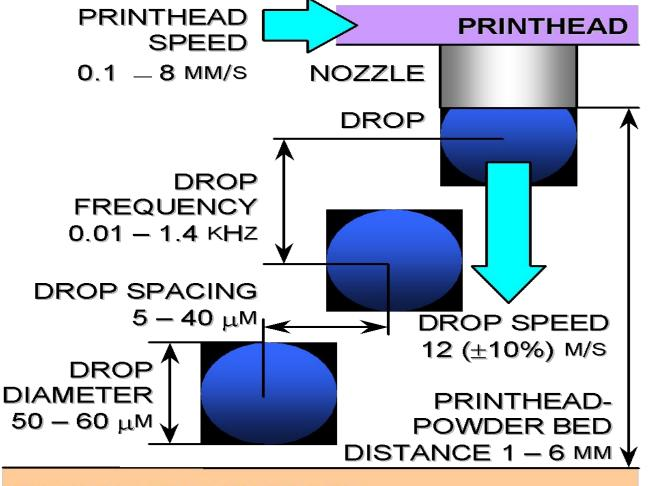
The Step Method for the Drop Speed
