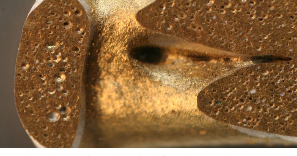
Sample Section. High porosity. Bimodal Pwd+AuSn. Inf. Temp.: 394°C
