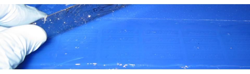
Cast material: Bi-component Urethane from SmoothOn Task 9 Degassing in vacuum @ 26" Hg for 5 minutes (working time)
