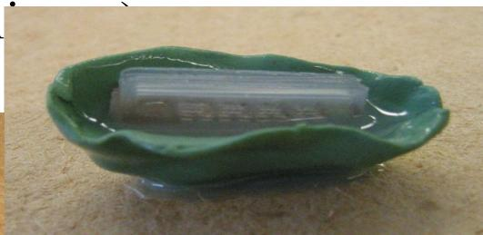
Cast material: Bi-component Platinum catalyst Silicone from Silicon Inc./Innovative Polymers P-20
