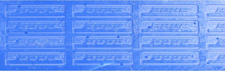
Depth of cavity: 750 μm (top two rows); 500 μm (bottom two rows)
