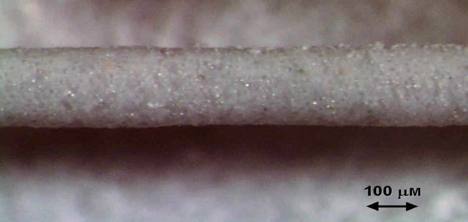
SEM image of a line made with 20 μm spherical with 12.5% wt. 5 μm equiaxial alumina powder; drop spacing: 10 μm
