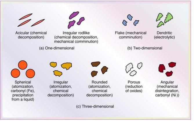
Particle shapes in metal powders, and the processes by which they are produced. Iron powders are produced by many of these processes.
