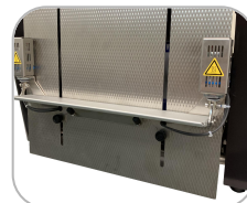
Articulating bag support for packaging heavy products
