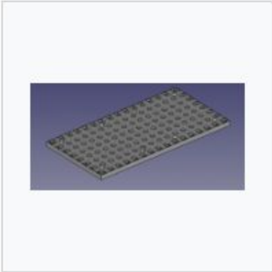
4x8x6.5" Insulated Exterior Wall File:Wall-4x8x6.5.fcstd
