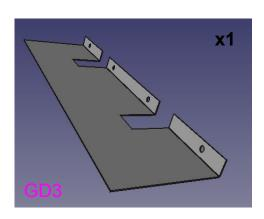
Perforate metal tails and bend upwards with a hammer and flat surface
