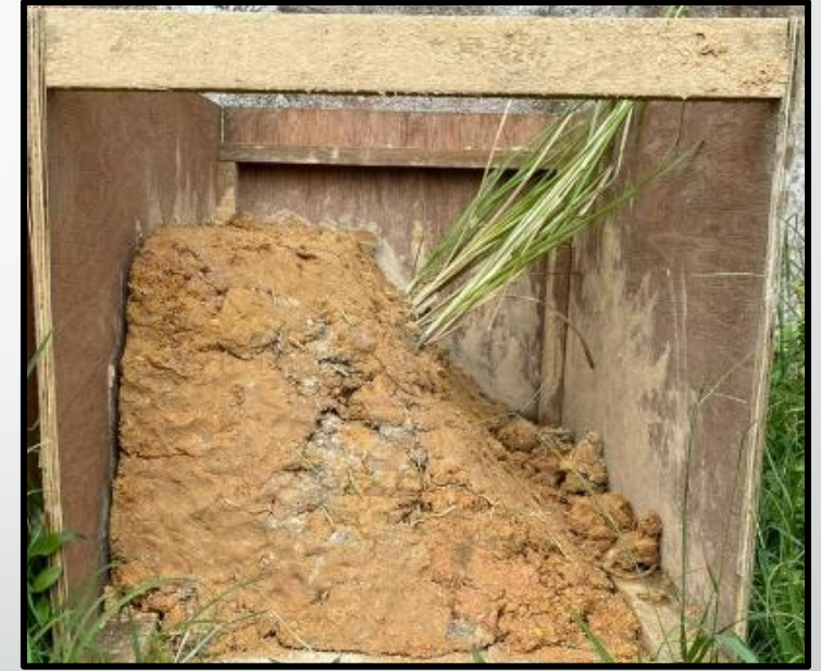
The design of soil modelling with the slope gradient of 60^\circ
