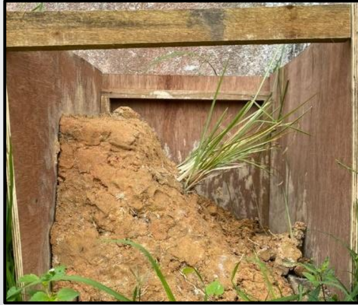
The design of soil modelling with the slope gradient of 50^\circ
