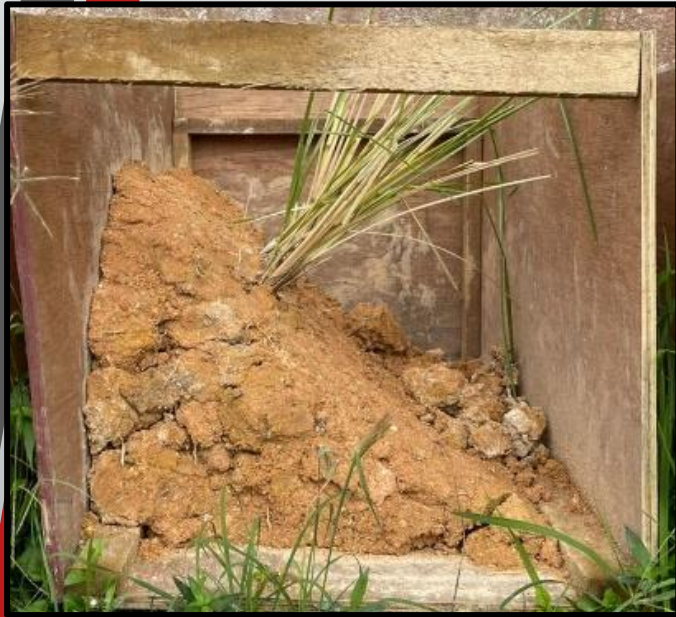
The design of soil modelling with the slope gradient of 45^\circ
