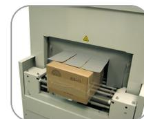
*Adjustable tunnel chamber height increases shrink efficiency*
