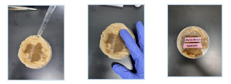
Pipette an additional 2 mL of liquid over the new paper disks (if needed, you don't want the seeds to dry out, but you don't want them to drown either!) and gently press down on the papers, enabling the solution to spread throughout the dish. At this point, the paper should be saturated to some degree. If the paper is not fully saturated, add more solution at your discretion, avoiding pooling. Replace labeled lid.
