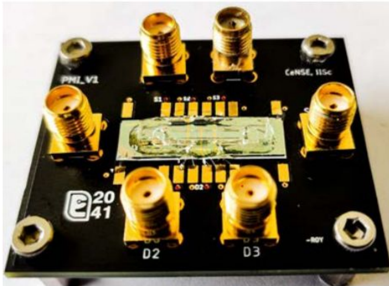
Figure 3: A PMUT-Microfluidic-Integration wirebonded to a custom-made printed circuit board
