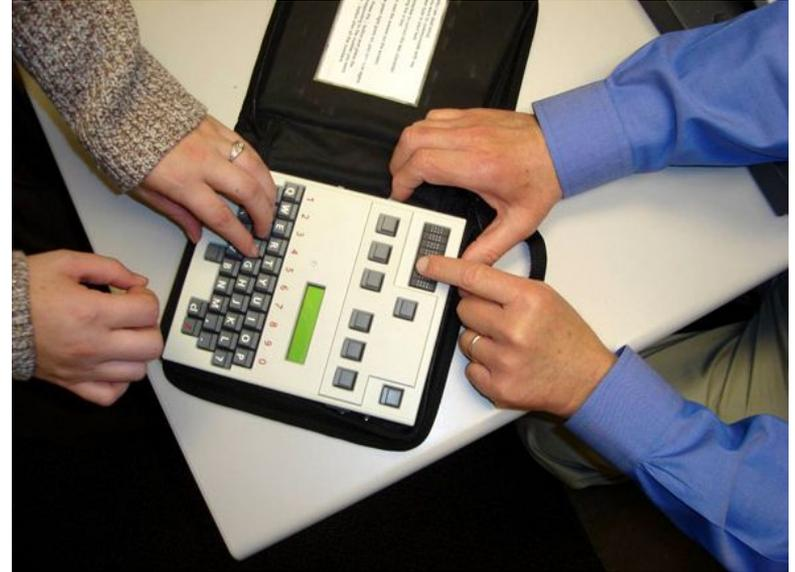
This photo shows two people communicating using a Screen Braille Communicator. The person on the left is typing a message on the keyboard. A person with deaf-blindness, on the right, is reading it on a refreshable braille display. Source: AADB, 2009
