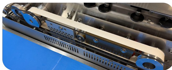
Heating and cooling bars and the V-belt used to transport the bags are easily accessed with the safety cover in the open position
