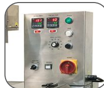
Simple to use controls adjust flow wrapping speed, sealing temperature, and more
