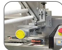
The standard film former manually adjusts to meet a range of package sizes
