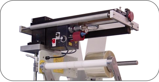
The FW 350T flow wrapper can be equipped with a date / lot code printer. Available with print orientation parallel to the fin seal or parallel to the end seal.
