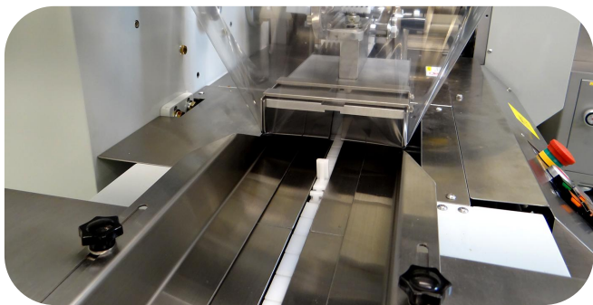
Delicate product conveyor with carrier card in-feed guide rails to handle product transitioning to the custom fixed former.
