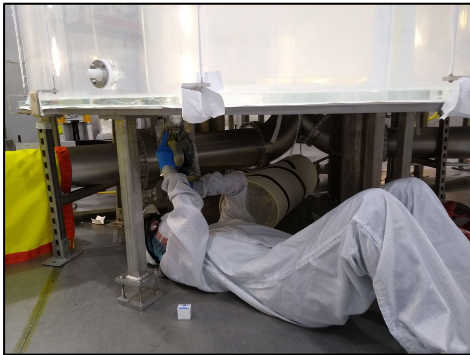
Alice installing the OCS fibres to monitor scintillator and acrylic degradation.
