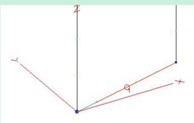
Expanded view of feed point. Ant is 5' off of the tower.
