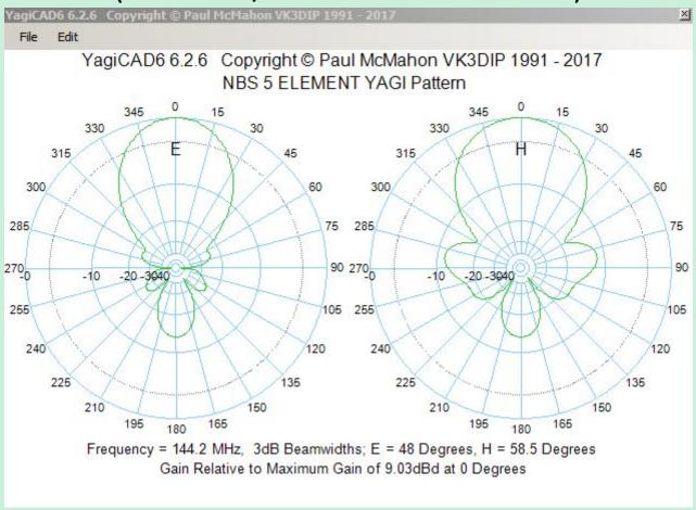
Pattern plots are most often shown in either the plane of the axis of the antenna or the plane perpendicular to the axis and are referred to as the azimuth or "E-plane" and the elevation or "H-plane" respectively.
