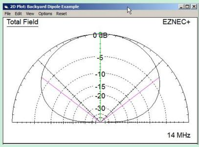
20 meter dipole at 30 feet. Not NVIS
