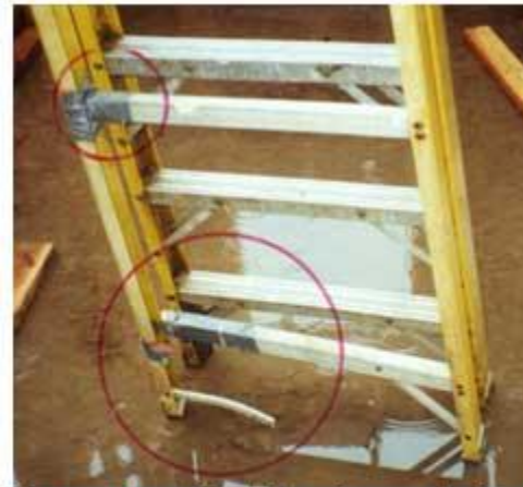
Do not use! Ladders in need of repair must be taken out of service immediately or replaced.
