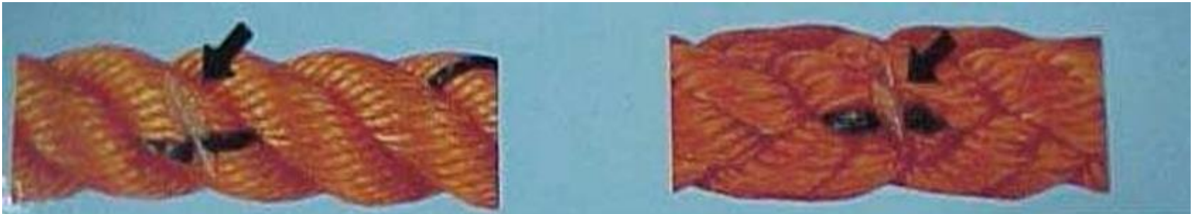
Damage due to spark or heat – surface damaged
