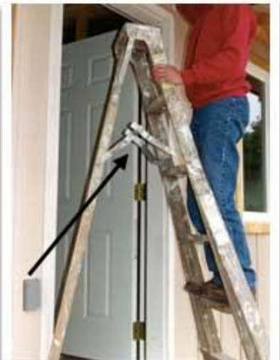
Danger! The spreader isn't fully open (WAC 296-876-40050).
