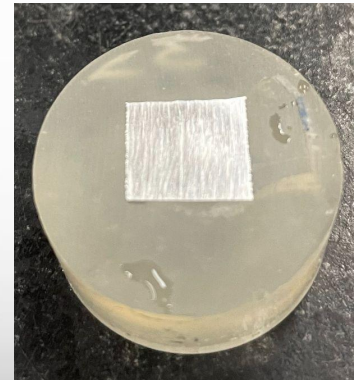
Ti64 sample in polymer mold (after grinding with 240 grit)
