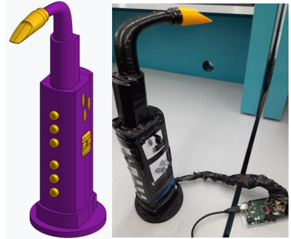
Figure 2. A CAD model of an electronic saxophone (left), later assembled and enclosed in 3D printed plastic (right).
