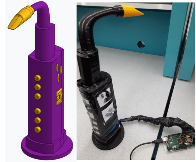
Figure 4. A digital rendering of an electronic saxophone (left), later assembled and enclosed in 3D printed plastic (right).
