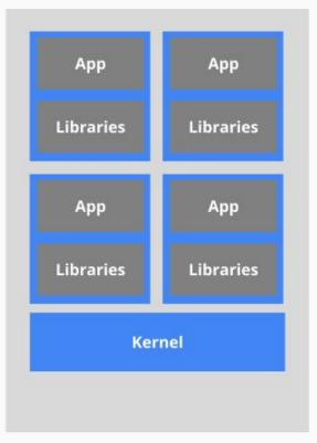
Heavyweight, non-portable Relies on OS package manager Small and fast, portable Uses OS-level virtualization
