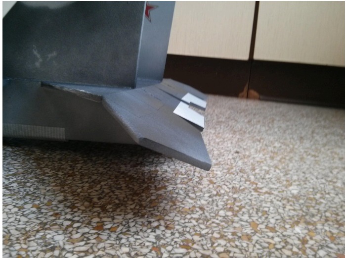
Control Surface Check Model viewed from port side, forward is left in pictures Left: Full Up Elevator; Right Full Down Elevator.
