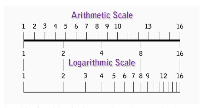
The arithmetic and logarithmic scales for numbers up to 16. The higher you go on the arithmetic scale, the more the logarithmic scale gets compressed.
