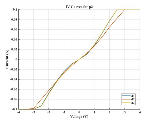
It appears that annealing at 250C was not enough to make the contacts ohmic, as it was for the Aluminum chips. Additionally, the contacts in these chips do not follow the usual trend of increasing resistance with increasing distances. Further annealing at 450C might provide more insights into this behavior.
