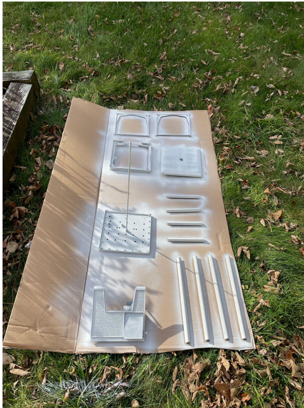
[Photos: Washing the machine & all of the parts laid out to dry before priming]
