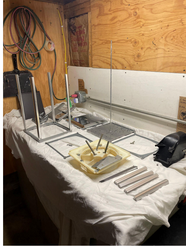
[Photos: Washing the machine & all of the parts laid out to dry before priming]
