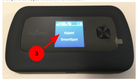
4. Press the top button (marked "MENU") to move through the hotspot settings.
