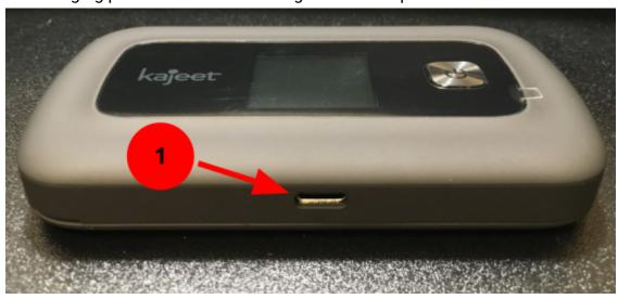
2. To turn the hotspot on, press and <u>hold</u> the power button **U** on the front of the hotspot until the screen reads "**WELCOME**".
