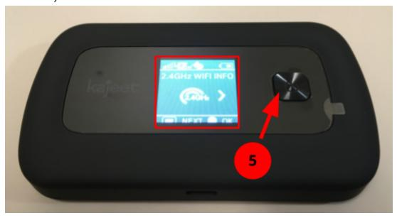
6. The wi-fi network name is the name scrolling across with the wi-fi icon next to it. The password is the word and/or numbers with the lock icon next to it.
