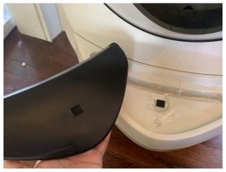
Next, I cut a piece of polycarb and attached it to the little vertical tabs of the drawer using VHB.
