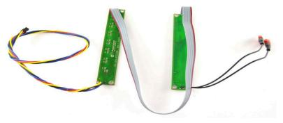
This version already has holes in the corners of the PCB, so you can just use a standoff to connect the two boards together with those holes.
