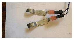
STEP 2: Tape the leads together with electrical tape
