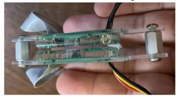
Make sure to leave a little bit of space between the sensors, as shown below.
