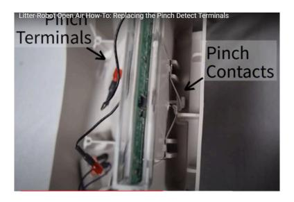
STEP 2: Connect the two ends of the wires together. Some ways to do this:
