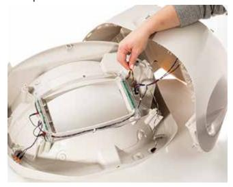
STEP 2: Connect the emitter and detector side of the sensor together using standoffs and screws.
