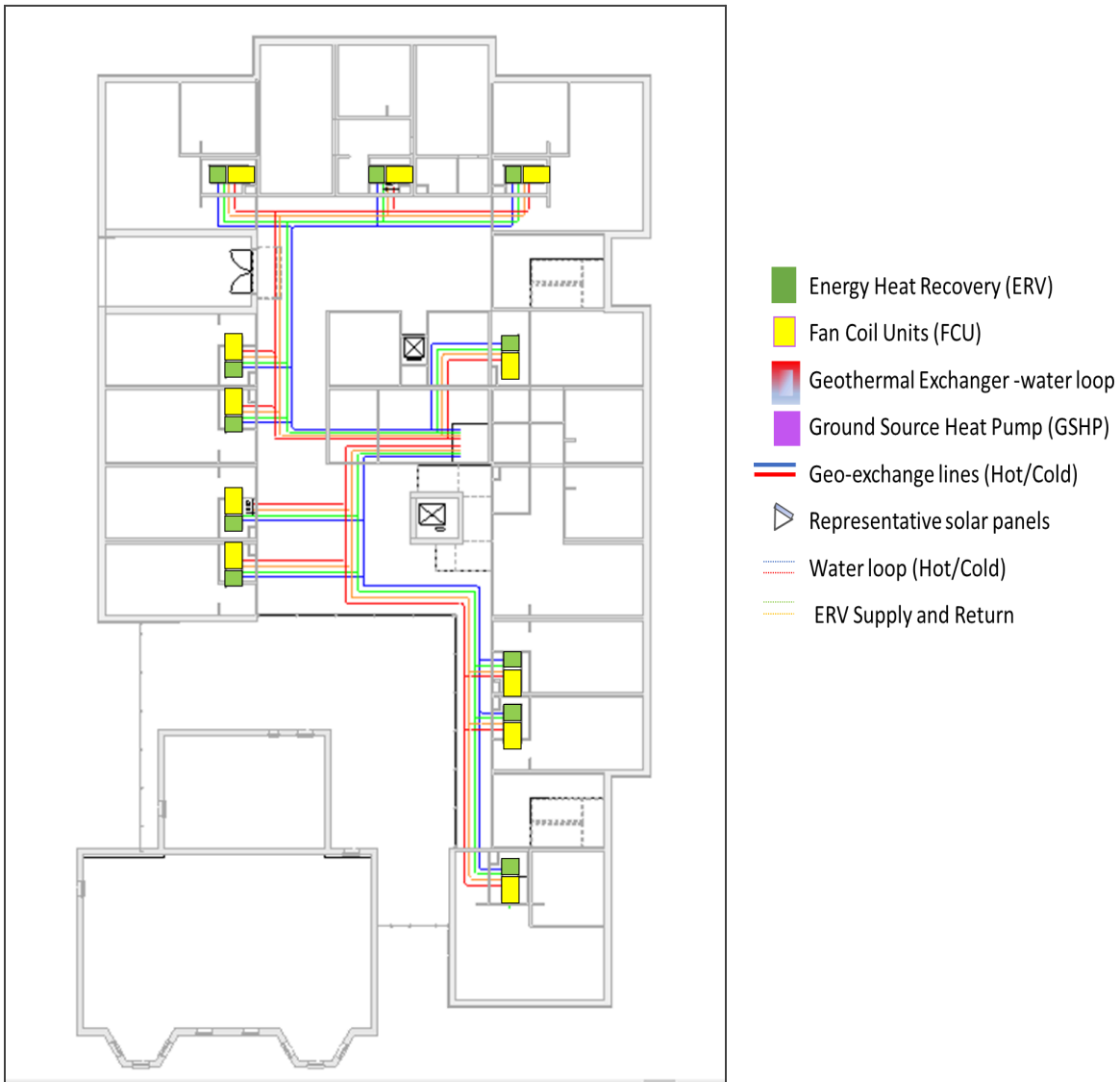
Figure 65: HVAC System- 1st & 2nd floors- GSHP & In-suite ERVs
