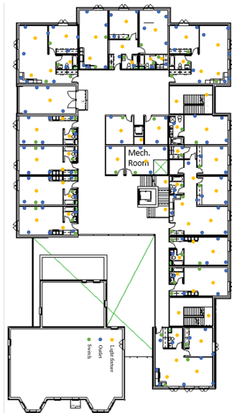
Figure 68: Approximate electrical layout for the first and second residential floors
