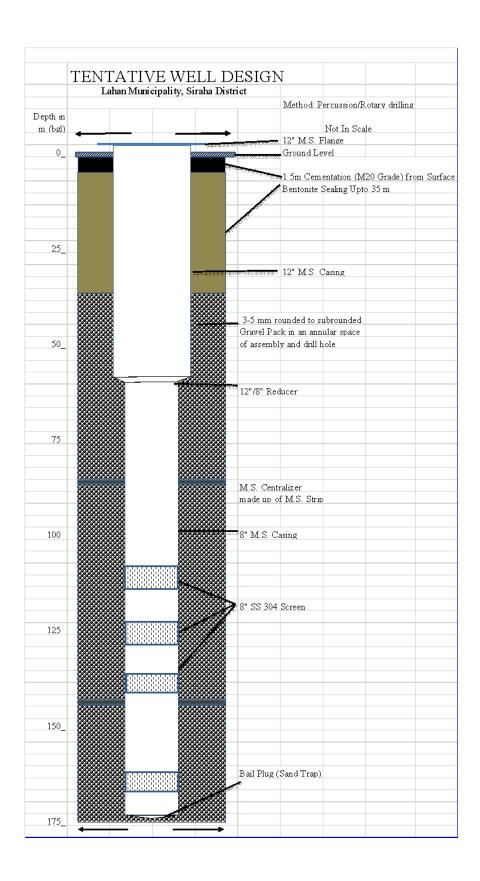
Drawing 2 – Typical Wellhead Design
