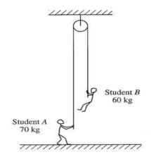
Two students are practicing rope tricks. They use a light rope and a frictionless pulley. Student *Albert* pulls on the rope and remains on the floor. The rope goes over the pulley and the other end is held by student *Bob*. What happens to the surface force of the floor on Student *Albert* when Student *Bob* climbs up the rope at a constant acceleration of 0.25 m/s²?
