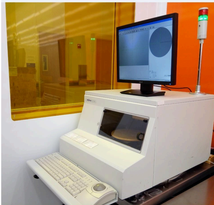
Figure 1 The P16 profiler, located in Keller Hall-Bay 1.
