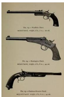
FIG. 15.—Guthrie-Ross Patent. match barrel, weight, 2 lbs., 8 oz.; 44 cal.
