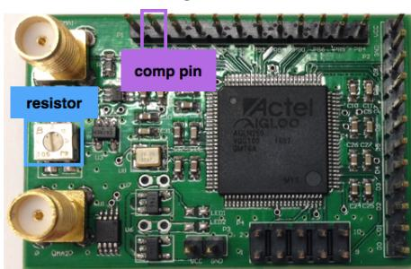
3. Download the codeword translator program into the FPGA using the programming header (yellow module). You need to be a bit careful when you connect FlashPro 5 programmer with the FPGA programming header. Make sure that your connection is
