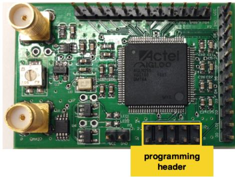
4. Download the ECG sensing firmware to the ECG sensing board.
