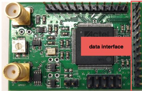
6. Connect two 2.4GHz antennas on the SMA port (blue module).
