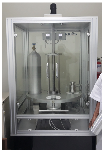
Figure 4. Automatic weighing system (AWS) for the preparation of biogas reference material in accordance with ISO 6142-1:2015 [26] . (TNR11, 1.15 space)
