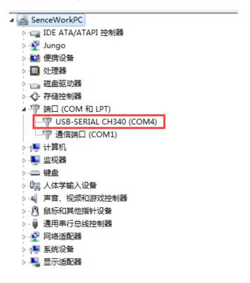
If you can not find out the right port to connect the robot, you need to install the driver to connect again.
