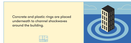
Fig. 6: The concrete and plastic rings around a building that redirect the seismic waves of earthquakes. Source: [17]
