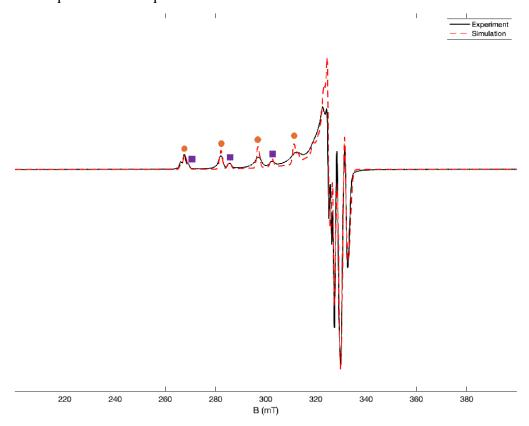
In this sample of a square planar Cu(acac)<sub>2</sub> derivative, the compound was sometimes axially hydrated and sometimes not. The parallel peaks corresponding to each species are marked in the spectrum with circles and squares respectively.
