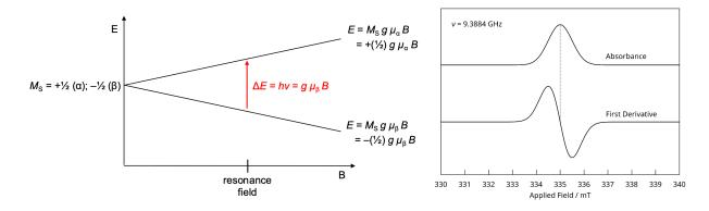
Typically, the CW EPR spectrum is reported as a derivative of the absorbance spectrum, because the measurement is performed using field modulation, which improves the signal-to-noise ratio. There are multiple microwave frequences at which one can measure CW EPR, but the most commonly used techniques are X-band (10 GHz) and Q-band (35 GHz).
