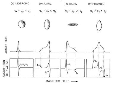
From here, change  $g_{\parallel}$  and  $A_{\parallel}$  to align the parallel features, and then move on to fitting the perpendicular features, following the steps explained above.
