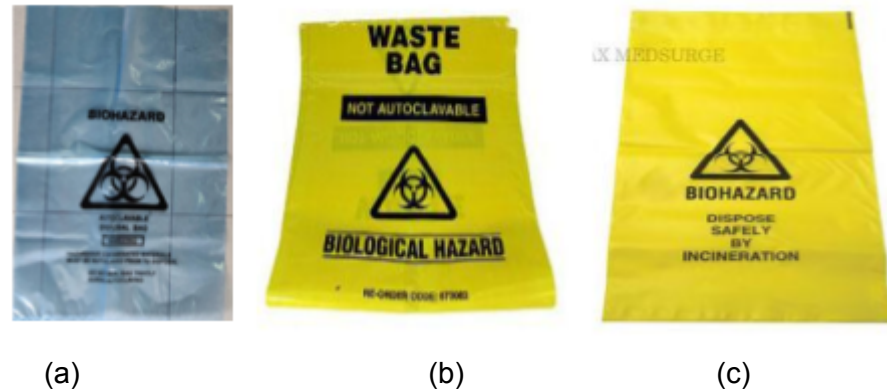
Figure 2 (a) is an example of Autoclavable bag, (b) and (c) are examples of incineration bags not suitable for autoclave.
