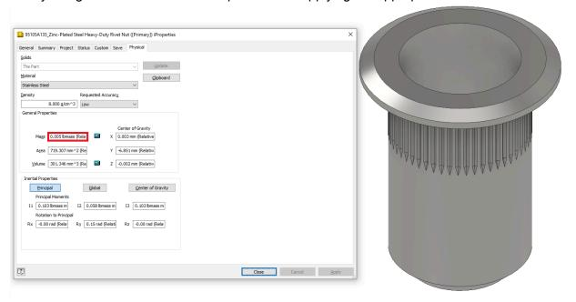
Since the mass of a regular rivet nut is 0.005lbs, you can edit the mass of the installed rivet nut you modeled to also be 0.005lbs. This level of accuracy is very rarely needed, and is usually more effort than it's worth, considering the fasteners are one of the lowest-weight parts of the robot.
