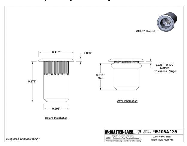
A 10-32 Rivet Nut from McMaster-Carr, with a drill bit size of 19/64" (0.2698")
