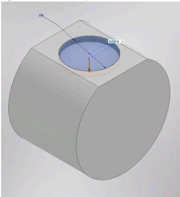
Then match the chamfer by making a revolution that will form a chamfer to guide the heat-set insert into its position, using the angle measured in CAD.
