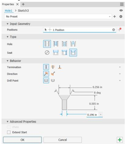
Major diameter (e.g. .256") — the "For Max Hole Diameter" specification + 0.01" Taper (e.g. 8°) — "Taper Angle" on Product Detail Total hole length (e.g. .505") — "Installed Length" × 1.5 Minor diameter (e.g. .196") — The close fit for the screw size
