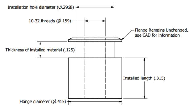
Finally, if you want to be more accurate about the mass of these modeled installed rivet nuts, adjust their mass such that they have the same mass as an uninstalled rivet nut, which you can find by using the uninstalled rivet nut part file and applying the appropriate material.
