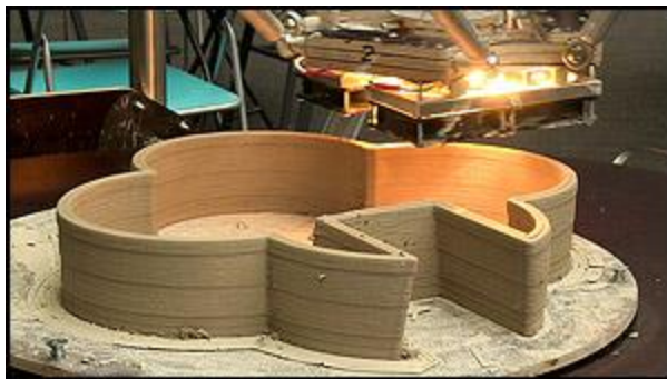
A WASP Big Delta 3D printing in clay, and a Robots in Gastronomy food printer
