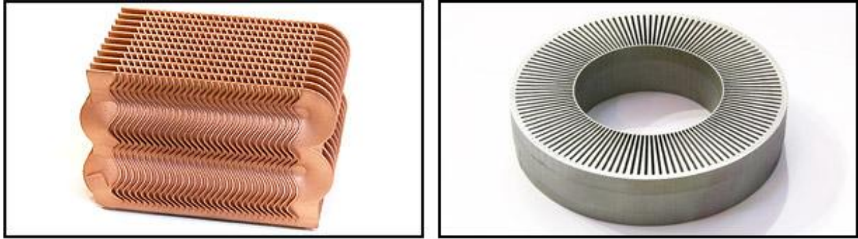
Final metal parts 3D printed via powder bed fusion
