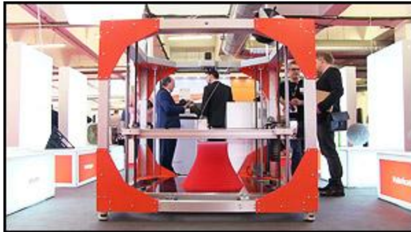
A BigRep ONE material extrusion 3D printer, and a table it has printed out.
