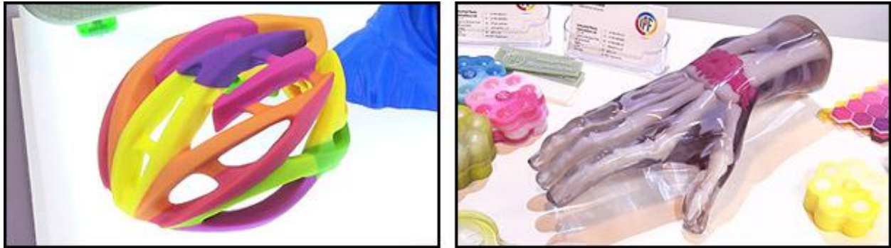
Objects 3D Printed on Stratasys "PolyJet" Material Jetting Hardware
