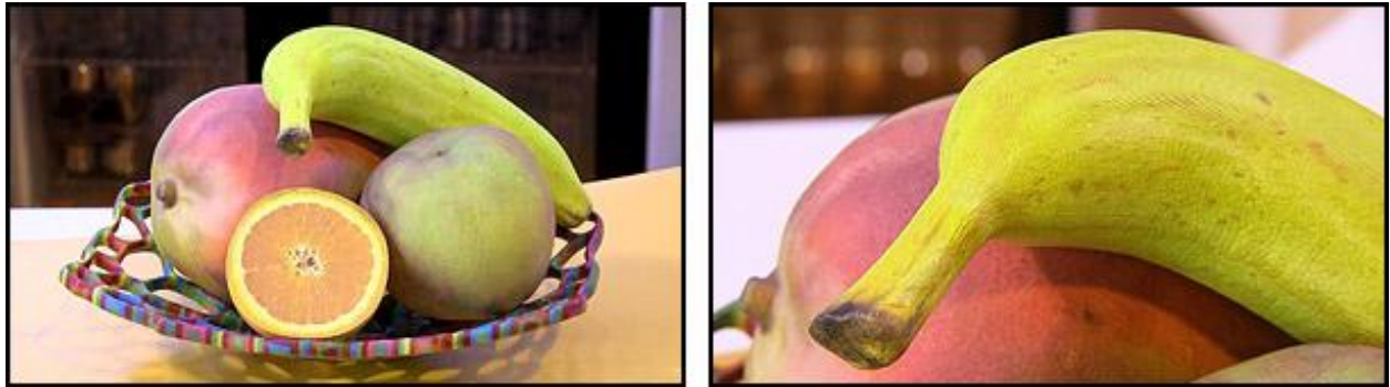
Fruit and bowl 3D printed in paper using an MCor sheet lamination 3D printer
