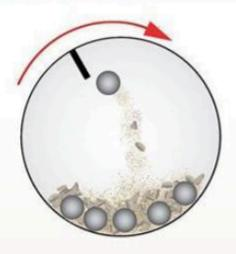
The Los Angeles Abrasion machine rotates at 30-33rpm, and is shown here with the shelf plate catching and dropping the aggregate sample and abrasive charge to the other side of the drum. This creates an impact-crushing affect. Aggregate sample and abrasive charge then roll within the drum creating abrading and grinding action. This action is repeated for 500 revolutions and degradation is determined as a percent loss of mass during the process.
