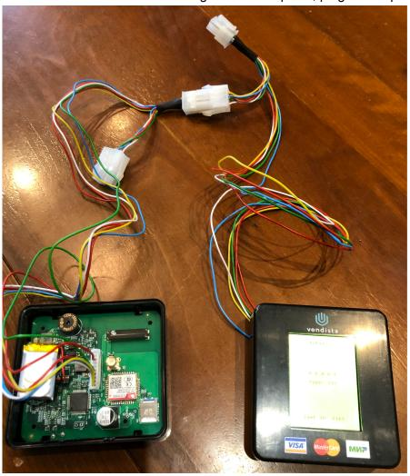
2. Supply 5 - 60V power supply to a free MDB connector. This can be done, for example, via the circuit board of the dispenser. Any MDB cable with a splitter can be used for this purpose, but the signal cables on the splitter should be cut off, leaving only the power cables.
