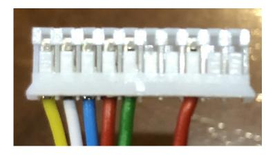
This is easily done by bending the plastic latches with a knife or screwdriver
