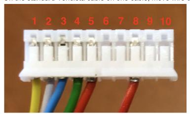
On the other cable, move wire 6 to plug 5, wire 7 to plug 4.
