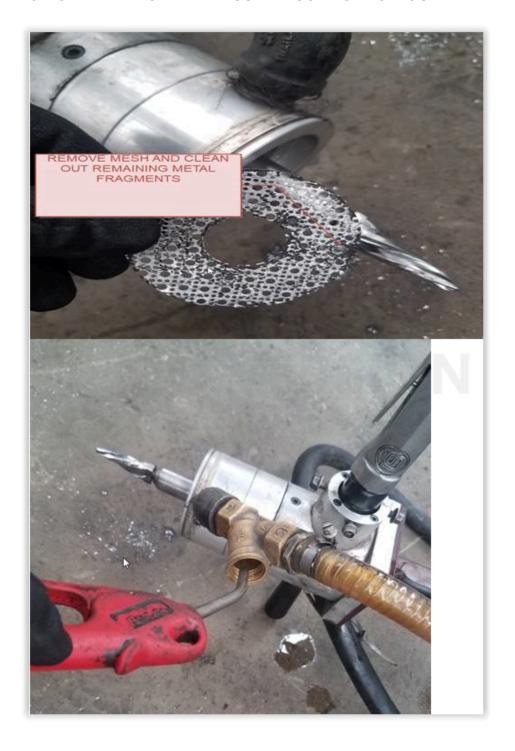
REMOVE FILTER BOLT WITH ADJUSTABLE SPANNER THIS SHOULD ONLY BIT HAND TIGHT REMOVE SHAVINGS AND RE-TIGHTEN
