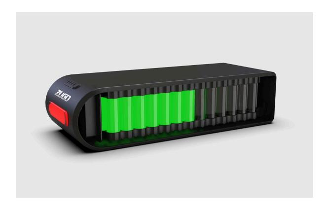
Lithium-ion batteries self-discharge, so storing the battery at 40%-50% (approximately 3.8 volts per cell) for an extended period of time is critical. Over-discharging the battery during storage causes an irreversible capacity loss or copper shunts to form on your anodes.
