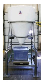
The existing method for adding the pulverized polyethylene powder to the rotational molding machine was to scoop the material by hand from the Gaylord containers into small, 7.5 gallon fiber drums. This method was slow and physically demanding. As material was removed from the Gaylord container, reaching the bottom with a scoop required dexterity and balance. In addition, the accuracy of using a scoop was oftentimes a problem.
