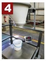
The dispensing system includes a custom two-part tubular steel dispensing frame. The upper part of the dispensing frame holds the bin and includes integral forklift slots to allow removal of the dispensing bin from the lower, base portion of the dispensing frame.
