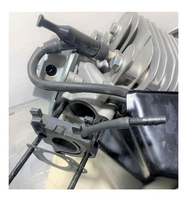
You will need to install the air filter adapter as shown below using the factory studs. It slides on the studs after the carb and gasket, use the lock nuts provided.
