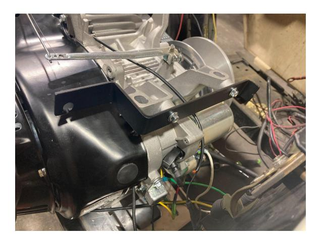
You will need to relocate the return spring so that it will pull the throttle arm back in the correct direction.
