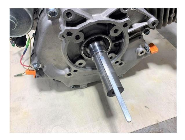
Apply a light coat of Anti-Seize lubricant onto the crankshaft to make future removal of the clutch easier.
