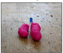
3. Place both wires from the battery pack into separate pieces of Play-Doh. Be sure the red wire is put in the piece with the long end of the LED in it.
