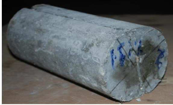
Figure 6: Concrete cylinder after splitting tensile test.
