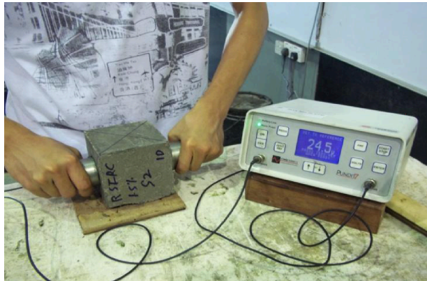
Figure 2: Testing of ultrasonic pulse velocity.
