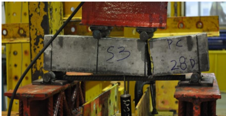
Figure 8: Failure mode of plain concrete beam in flexure.
