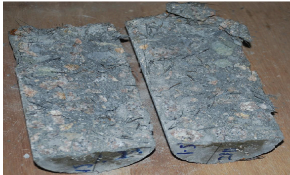
Figure 7: Distribution of steel fibre in broken cylinder.
