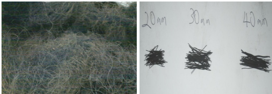
Figure 1: Recycled steel fibre before and after shredding
