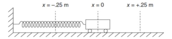
A lab cart of variable mass m on a frictionless surface is attached to a spring, as shown above. The rightward direction is considered positive. The spring is neither stretched nor compressed at position x = 0. The cart is released from rest at the position x = +0.25 m at time t = 0.
