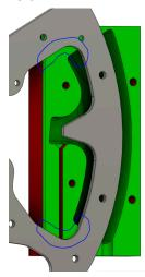
2. Clamping - my first attempt was to use vice grips, but that deflected the mold and made the process really hard. Second version I made 4mm holes true to the mold and used threaded rod, bolts and washers to clamp it, much easier.
