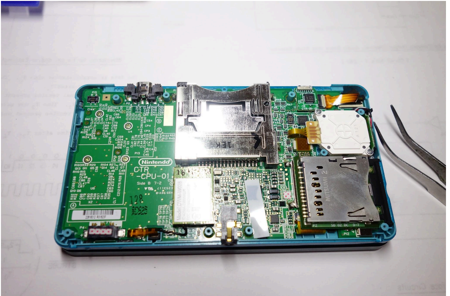
Now you can finally put the lower case away, the underside of 3DS's motherboard is now in full view.
