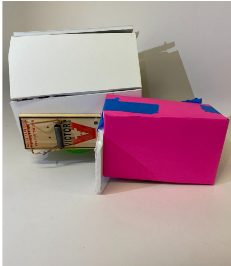
Figure 2. Rapid prototype where a mouse trap was used as a clip that would attach to the cross beams of a car.
