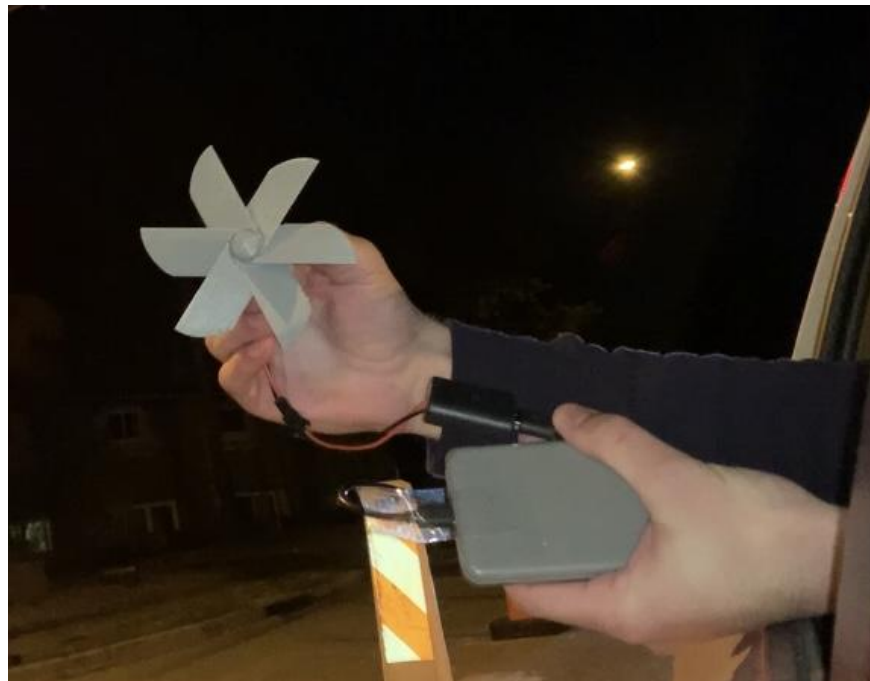
Figure 17. Initial energy generation component testing. The turbine blade and motor are connected to a battery, which lights up when it begins to charge.
