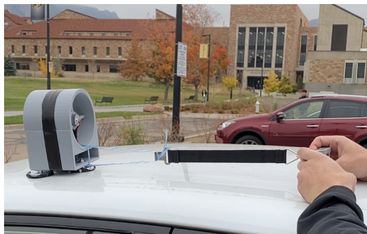
Figure 18. Testing for the mounting component in action. Tether is threaded around the base of the turbine and hooked onto a spring scale.
